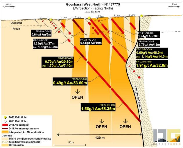
Figure 6. Cross-section Gourbassi West North Zone
